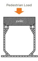
Jonite Mini Grate $^{\text{TM}}$  being installed on compatible channels. Grates come with recessed grooves for a snug snap and fit.
