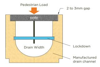
Install directly on the compatible drain channels. Some models can be bolted down with lockdown features.
