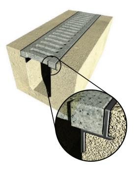
A 90-degree seating edge can be obtained in a variety of ways using L-steel angles.
