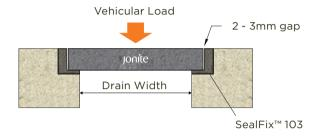
Jonite L-Trimmers™ is installed using dry fixing with SealFix™ 103 (epoxy mortar).
