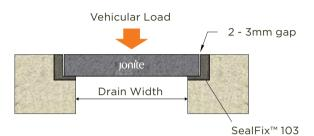
Jonite L-Trimmers<sup>™</sup> is installed using dry fixing with SealFix<sup>™</sup> 103 (epoxy mortar).
