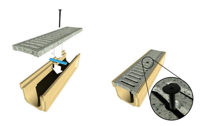
After placing the lockdown plate, a countersunk bolt is then bolted in to secure.
