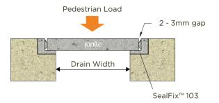
Jonite Stud Trimmers™ is installed using dry fixing with SealFix™ 103 (epoxy mortar).
