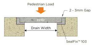
Jonite L-Trimmers<sup>™</sup> is installed using dry fixing with SealFix<sup>™</sup> 103 (epoxy mortar).
