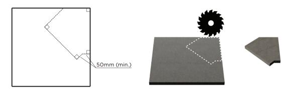
**IMPORTANT:** Supported length of the Grate Tile™ must be at least 50mm
